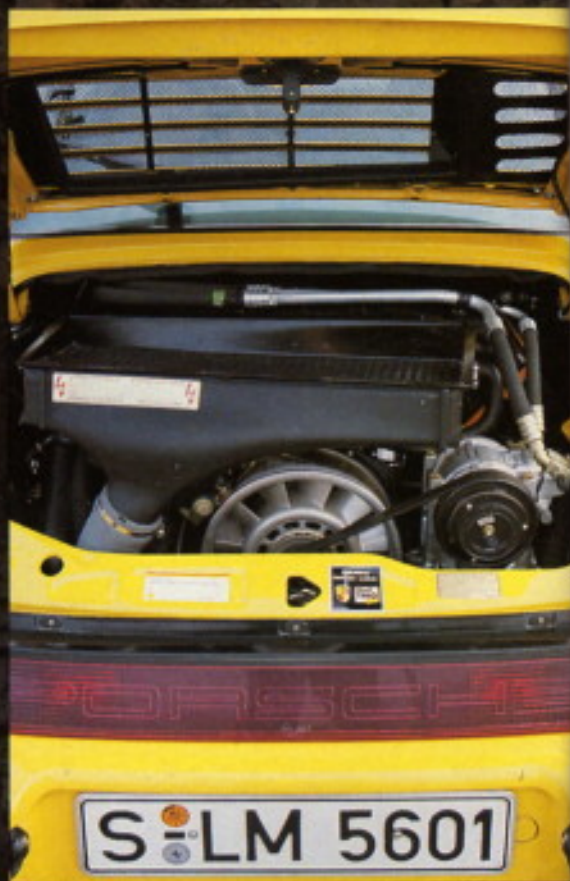
Carrera crankcase is the biggest change, but 360bhp Porsche turbo power requires very expensive innards
